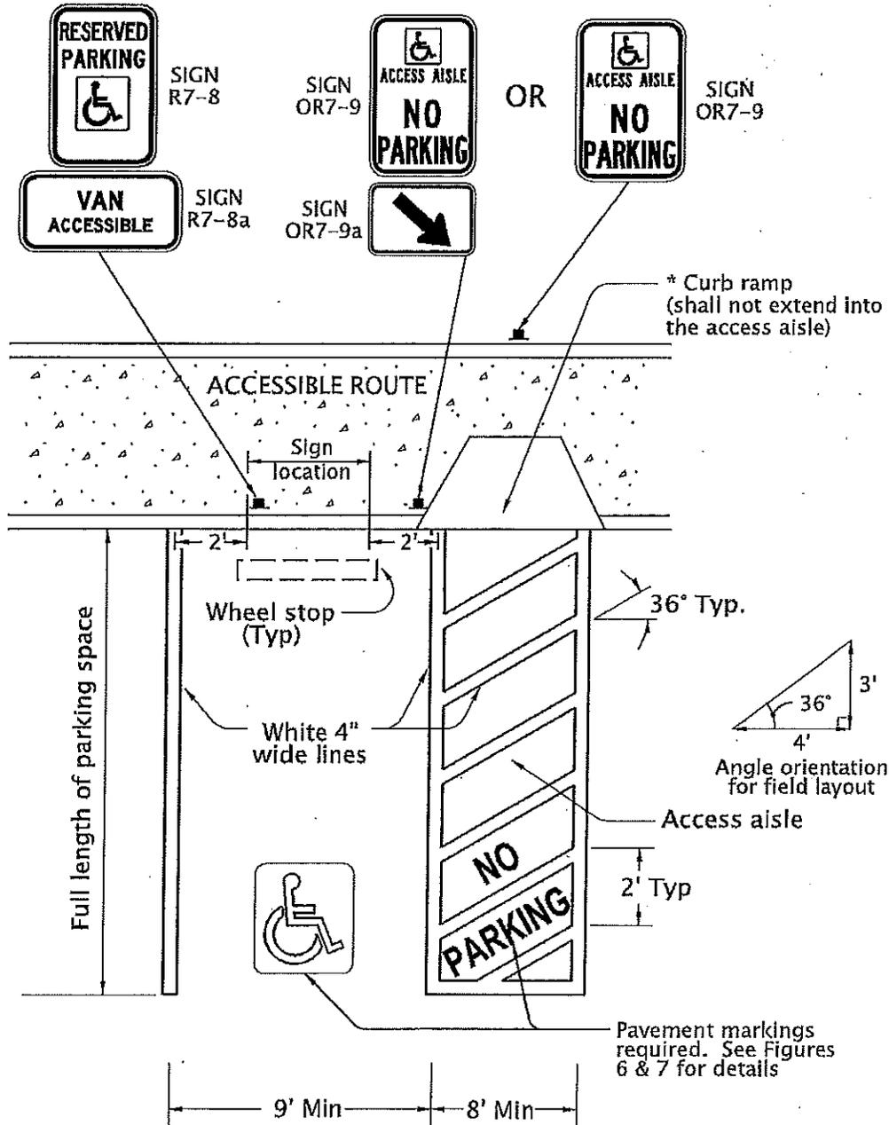
\* Detectable warning surface required if curb ramp is located within public right-of-way
