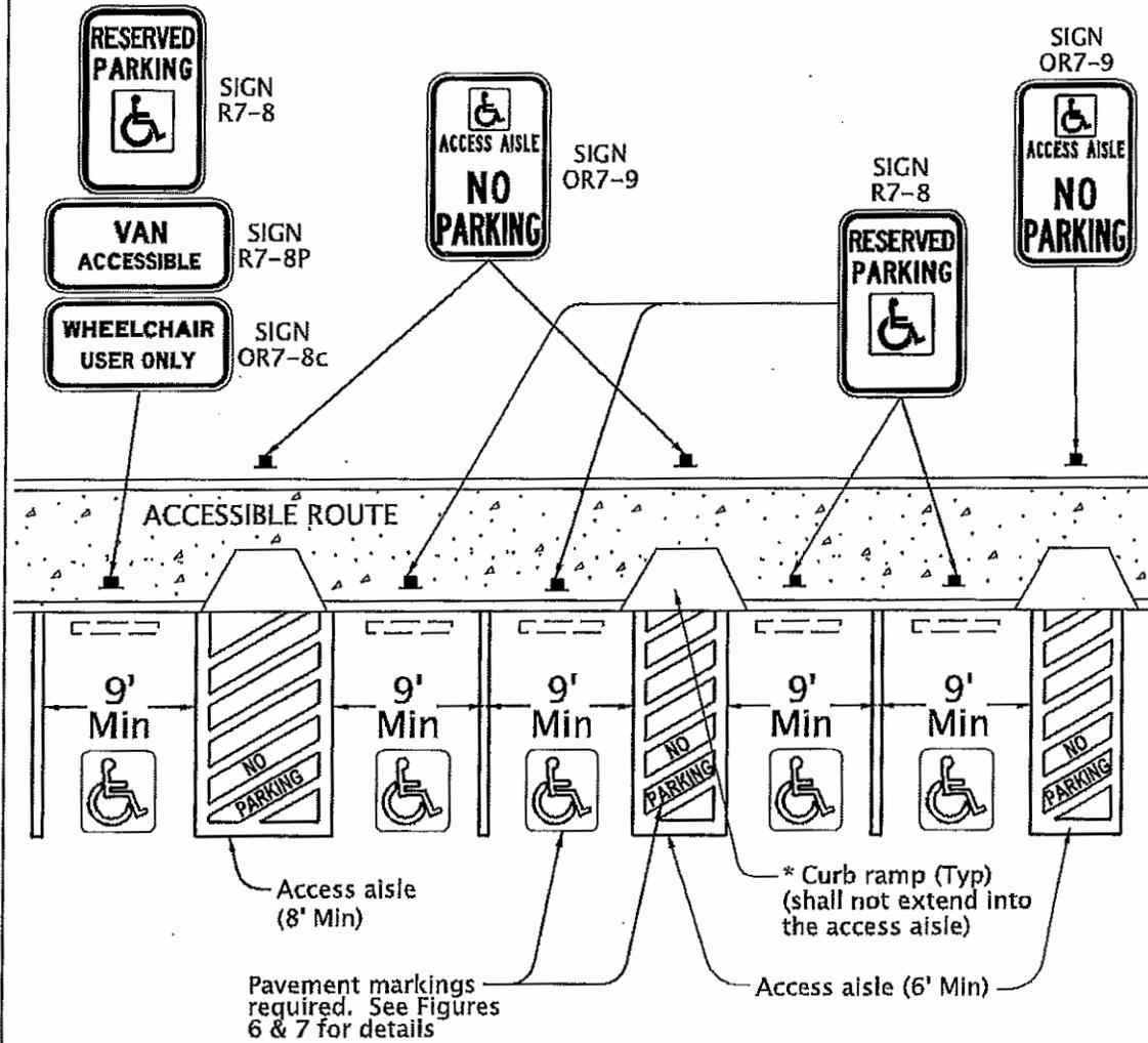
\* Detectable warning surface required if curb ramp is located within public right-of-way
